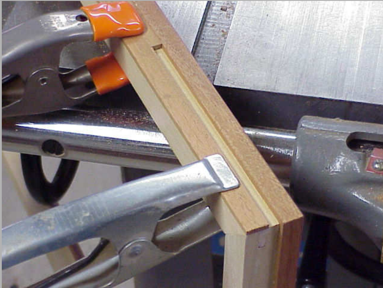
Gluing 1/8" Mahogany trim to cover frame sides.
