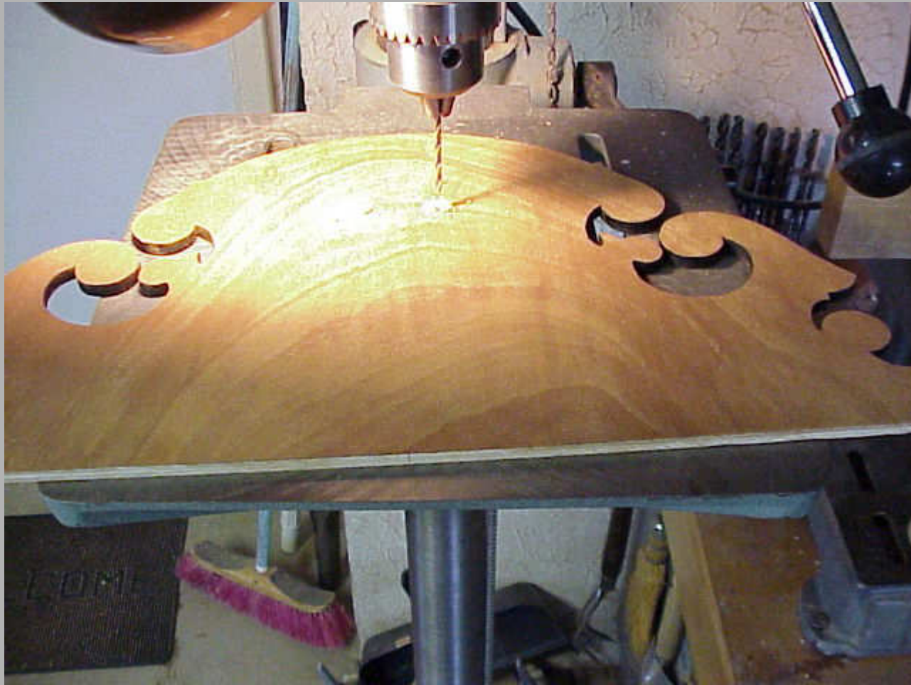
Holes being drilled in hood to fasten scallop shell.
