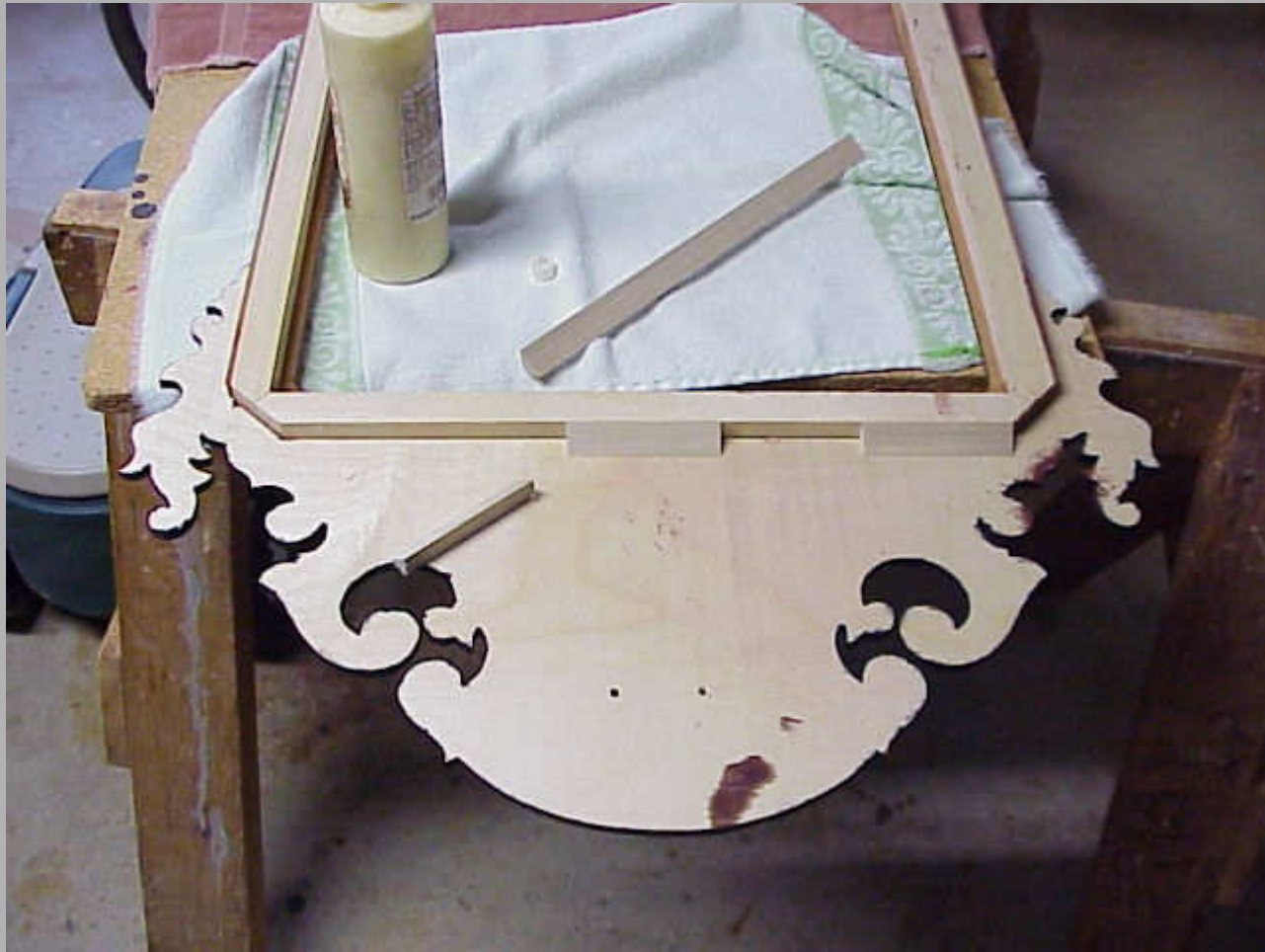
Support blocks being glued to frame & hood.
