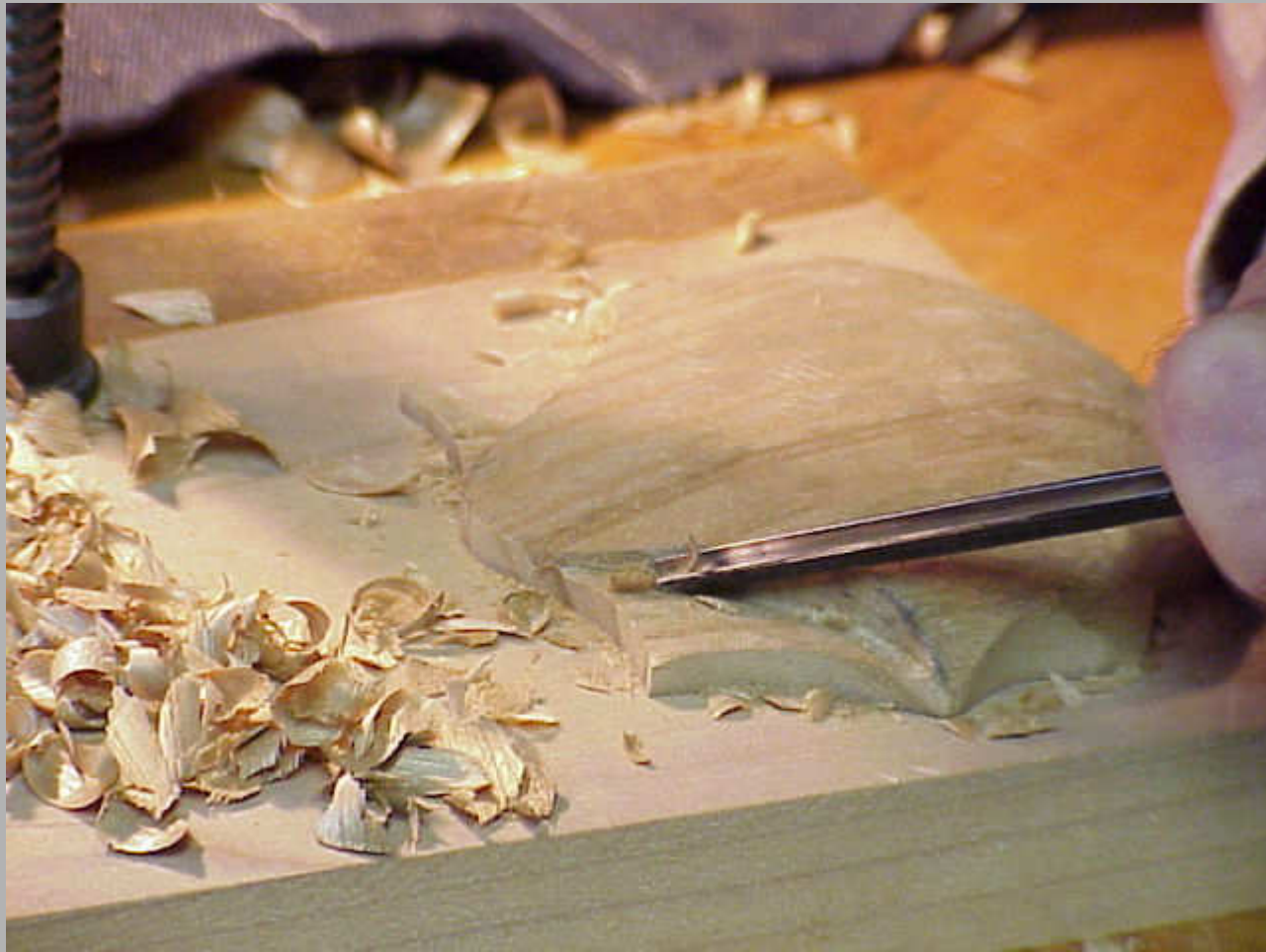
Carving veins in scallop shell wings.
