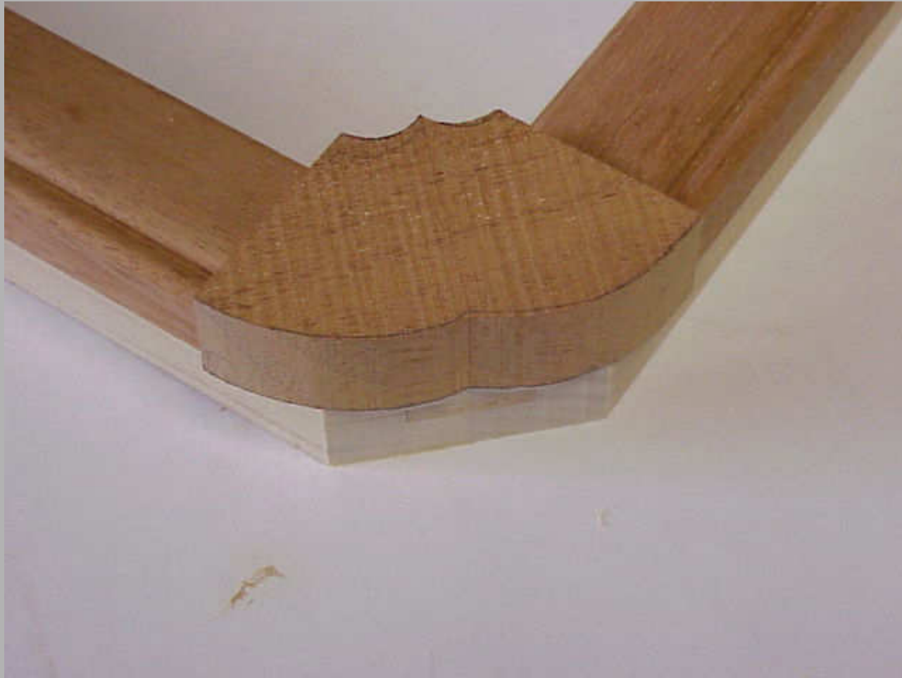
Corner block band sawn to shape.
