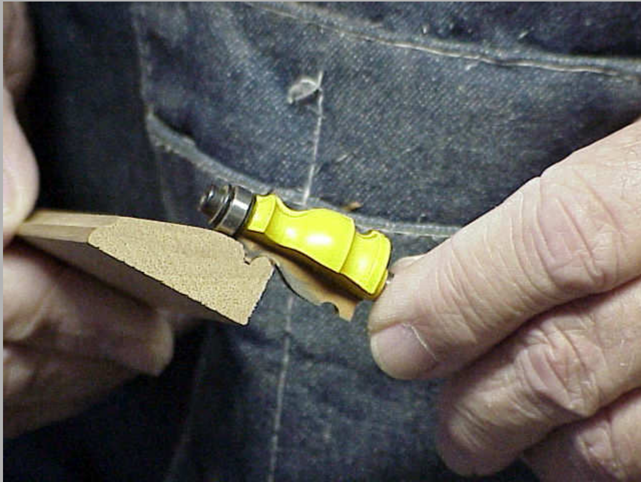
Shaper cutter used to form small edge beading.
