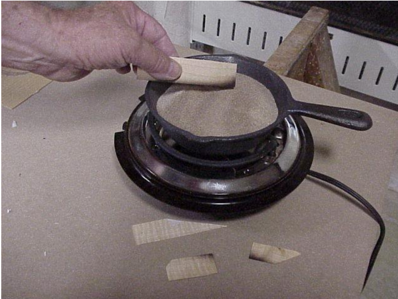
View of a ray after sand shading.
