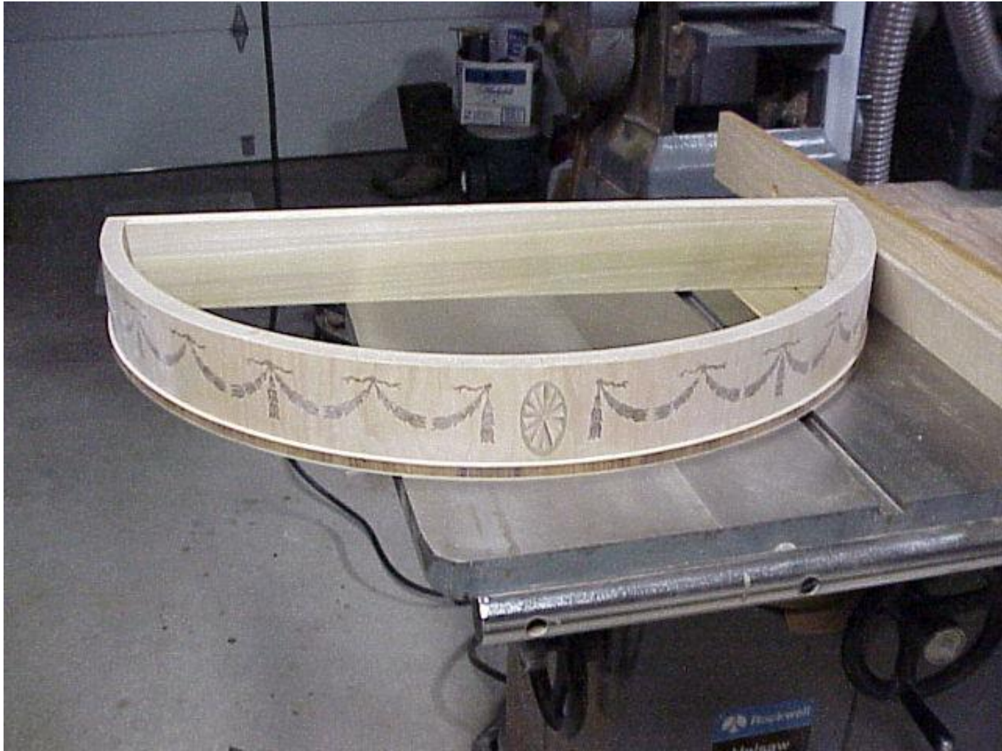
View of completed apron. Note: Use of a very fine blade & colored filler makes the cut lines invisible
