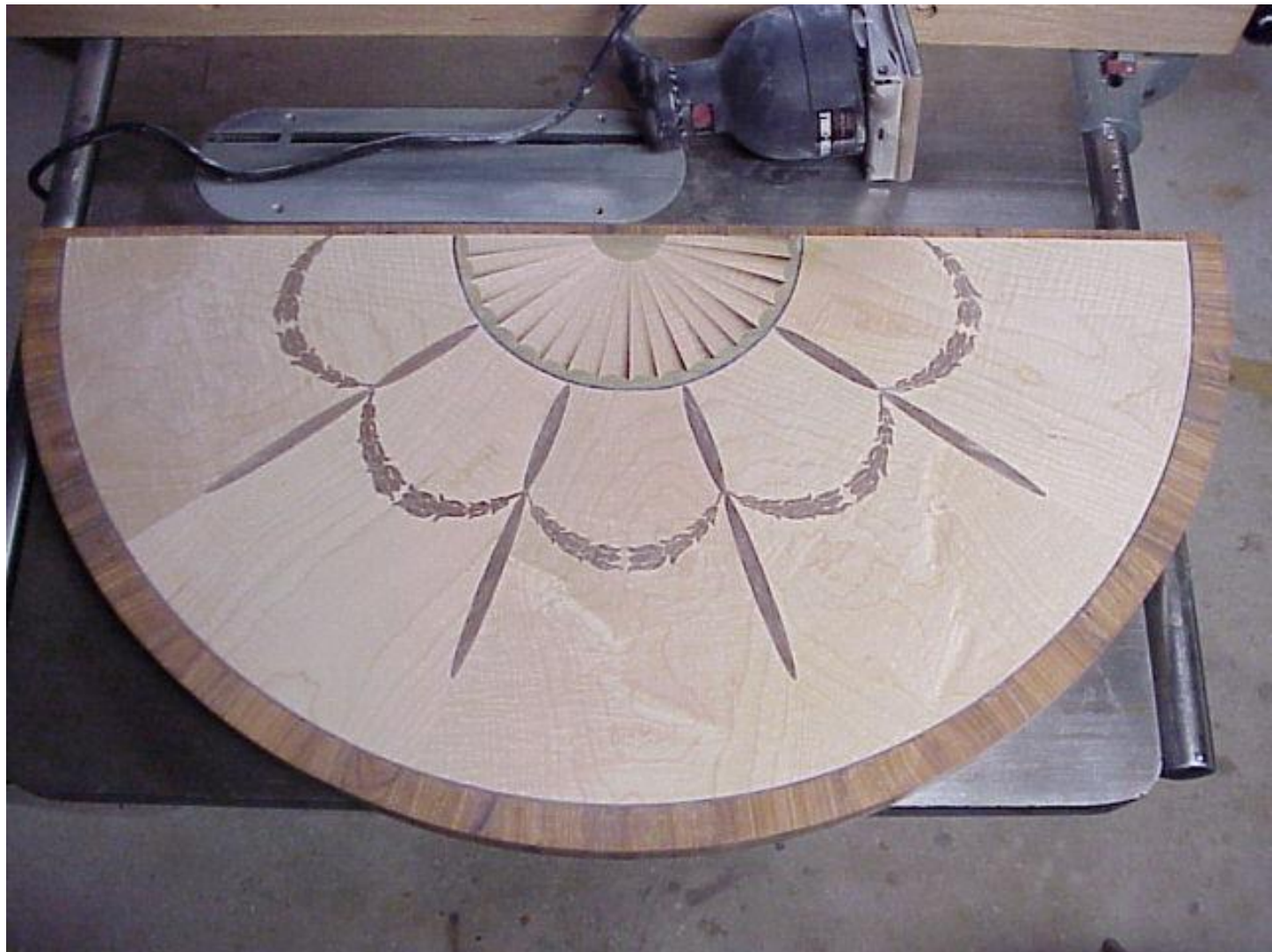
View of top after gluing, veneer tape removed and top sanded smooth.
