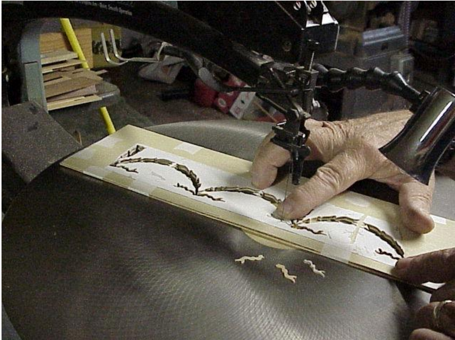
The veneer pad being cut on the scroll saw using an Olson #3/0 marquetry blade running at a low speed.
