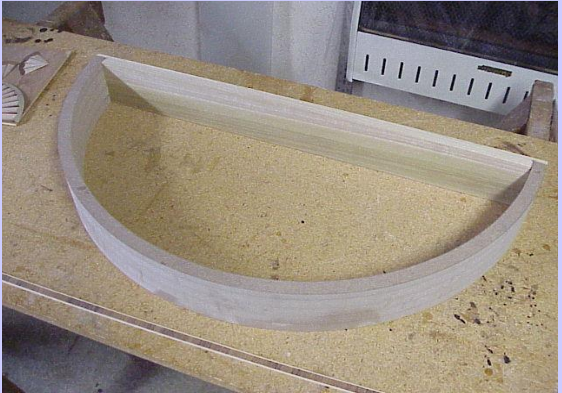
The curved apron is constructed of MDF and the back of Poplar.
