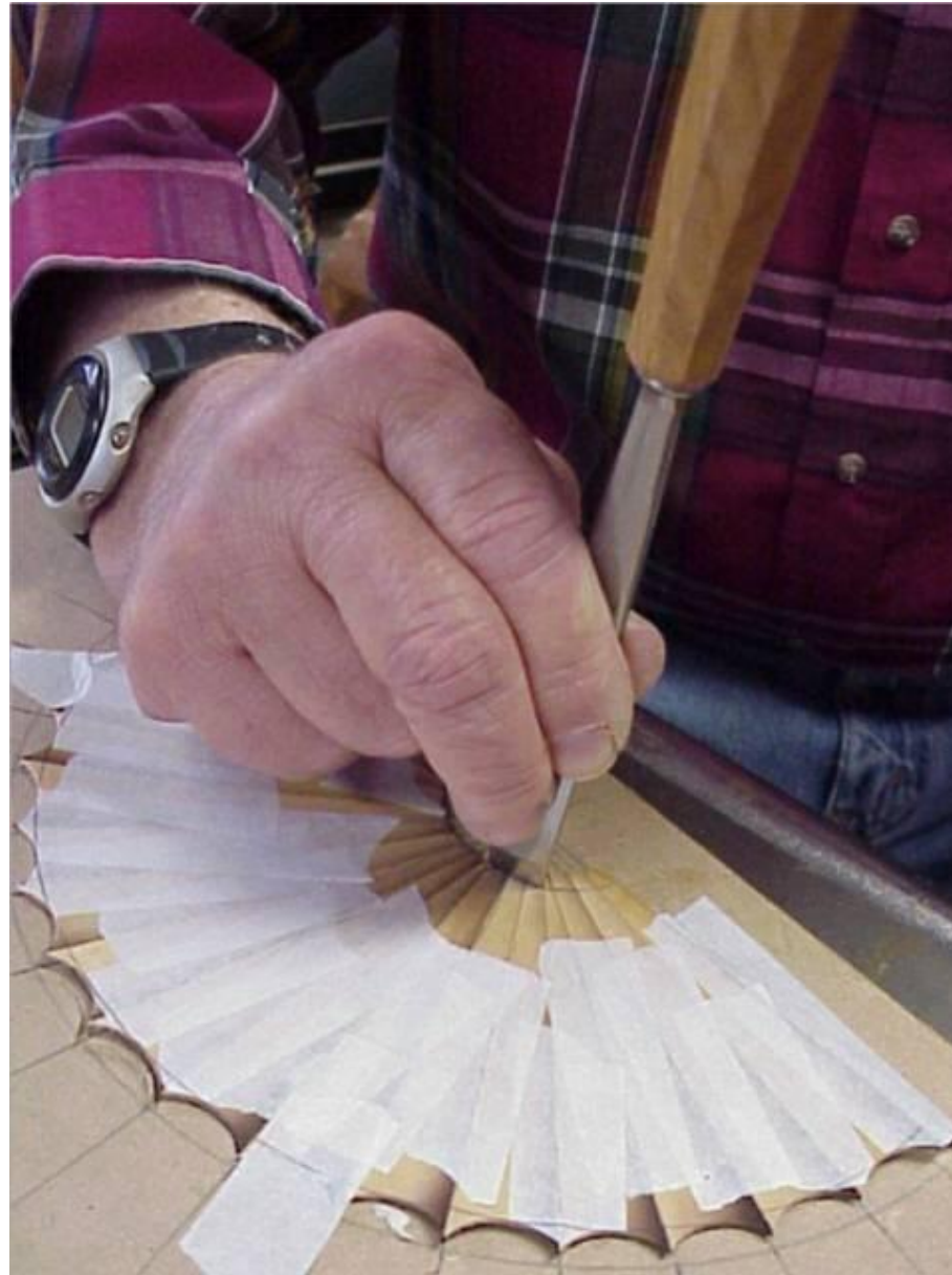
Chopping inside end of rays with a 3 sweep chisel
