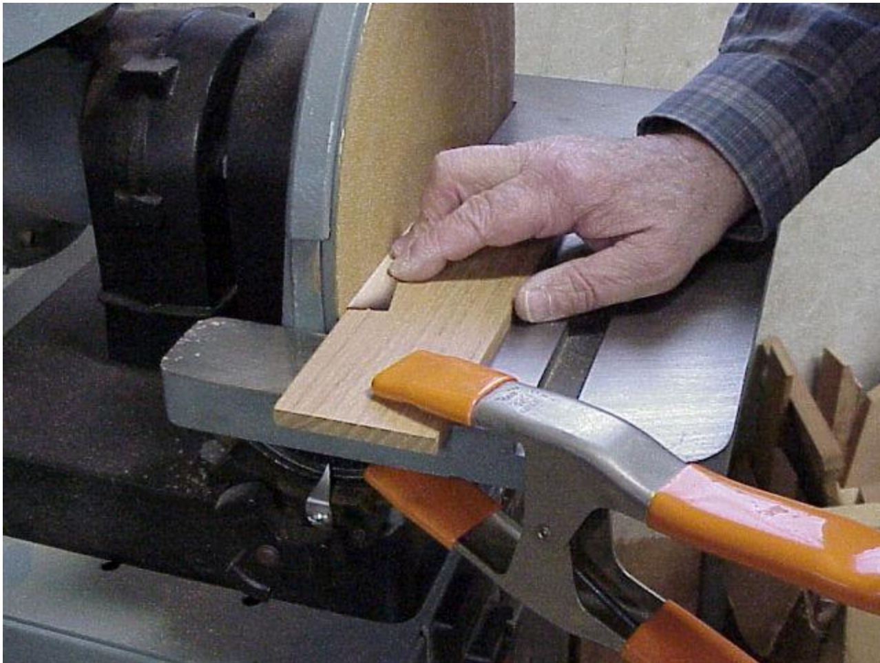
Sanding the cut edge of ray to straighten
