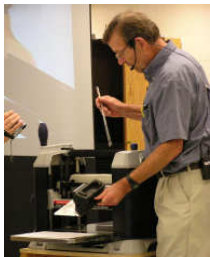
George Murphy Demonstrating the art of changing blades in a planer.
