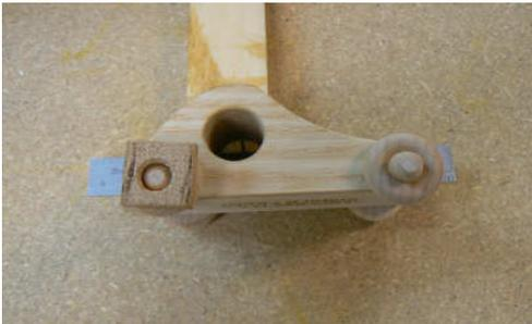
What appears to be a square wheel in above picture is a spacer, placed over the axle pin, on that side of car, to prevent that axle from being pushed in too far, while pressing axle pin from opposite side of car.
