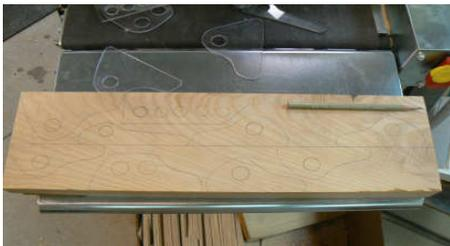
Set up drill press, with a wooden auxiliary table. With your choice of size of Forrester drill bit, for drilling the window holes. I use
