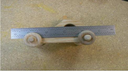
Repeat on other side, BUT, before placing hand clamp on, place square wooden spacer over axle on opposite side, to prevent that axle from being pushed in too far. Set aside for glue to dry, after making sure that you do not have any glue squeeze out that could glue the wheel to axle or side of car.
