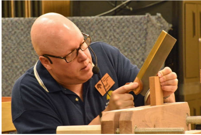
Paul Sanow demonstrating hand-cut dovetails
